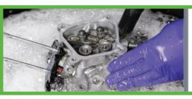
Heated to 42°C, the microbes become active in the ROwash solution and eat the oil and grease turning them into CO<sup>2</sup> and water – effectively recycling the fluid.
